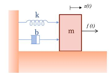
$$\frac{Y(s)}{U(s)} = \begin{bmatrix} \frac{1}{\det(sI - A)} \\ \frac{s}{\det(sI - A)} \end{bmatrix} = \begin{bmatrix} \frac{\frac{1}{m}}{s^2 + \frac{b}{m}s + \frac{k}{m}} \\ \frac{\frac{s}{m}}{s^2 + \frac{b}{m}s + \frac{k}{m}} \end{bmatrix}$$
